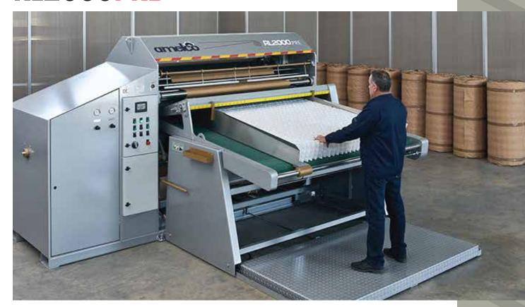
Suitable for Roll Packing very tall spring units of up to 22cm height. Fast & Easy to operate, NO special operator skills are required, minimal installation and training.
